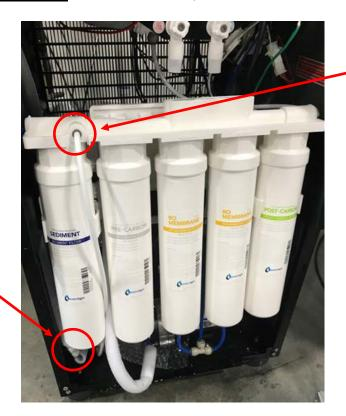
Disconnect, and plumb to drain for filter flushing.
