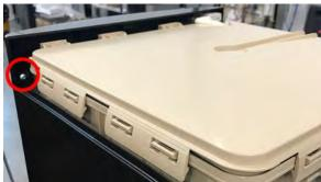
3. Remove the lower front panel to access the lower compartment. To do this, remove the two screws under the lower lip of the panel, then push down and pull out. The panel should hinge outward and be free to remove and set aside.
