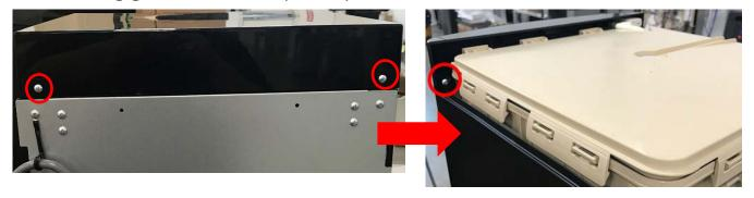
2. Once the front panel has been removed, the PCB shield must be removed. Remove the two screws on either side of the shield, lift, and pull away from the PCB. Be careful not to damage the PCB or any wires surrounding the PCB.
