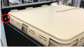
2. Remove the screws holding the back-silver panel in place. Remove and set aside.
