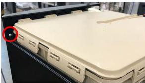
2. With the front upper panel removed, locate the white plastic ice chute. Locate the silver dispensing ring mounted to the bottom of the chute, protruding into the dispensing area. Twist this ring 1/4 turn counterclockwise and pull down to remove. Notice the four screws around the perimeter of the ice chute. Remove these screws. Trace the Ice Door Motor wire up to the PCB and remove if necessary.
