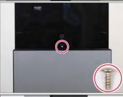
4. Press down on the Front Cover Lower Assembly and remove in the direction shown
