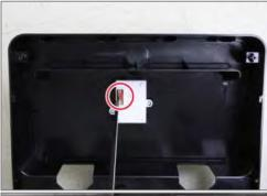
6. Remove the two screws (THT 4X12) from PBA Cover Front Assembly
