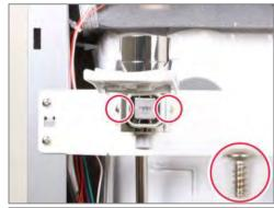
2. With a flathead screwdriver, remove the hose connected to the Hot Water Faucet Safety Assembly
