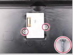
7. Remove the two screws (THT 4X8) from PBA Front Assembly
