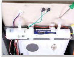
2. Remove the Ultraviolet sterilizer in direction shown.
