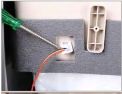
2. Remove the CTS Water Level P Sensor in direction as shown.
