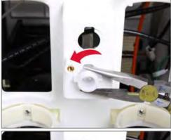
3. Line up the Hot Water Connector Drain Assembly to the groove on the Filter Bracket. Push it in the direction as shown with needle nose pliers.
