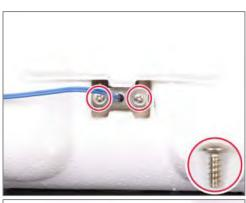
2. Remove the Cold Temperature Assembly Sensor in direction as shown.
