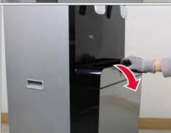
3. Remove the screw (THT 4X10) located on the Front Cover Lower Assembly as shown.
