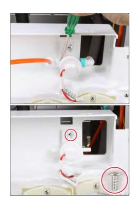
2. Remove the single screw THT 4x8 on the SENSOR-E LPS Assembly.
