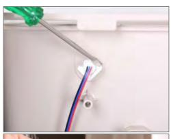
2. Remove the CTS Water Level N in direction shown.
