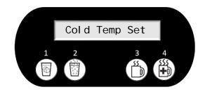
The cold temperature can be set between 3°C and 12°C (37°F and 54°F) depending on which units are selected (°C or °F) in the F/C programming setting.
