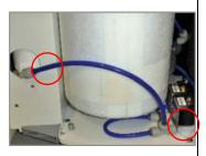
7. Attach new tube from Water Inlet to Tee at Solenoid. Care to be taken to ensure that the new tube does not touch the compressor, nor any sharp edges.
