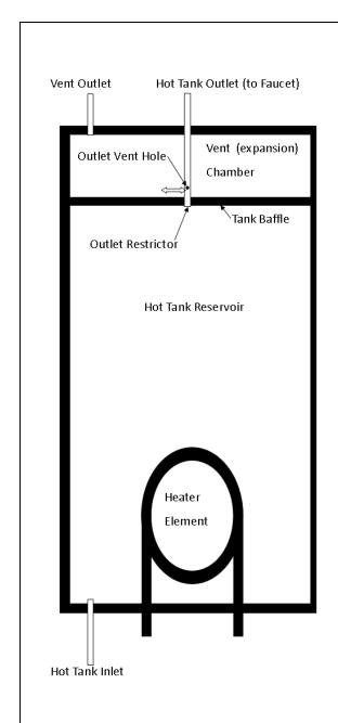
All *Waterlogic* Hot Tanks have a built in Vent or Expansion Chamber in the top of the tank except for WL270 (GF) units.
