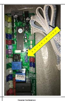
4. Turn the Hot temperature calibration counterclockwise from 12:00 position to 11:00 position
