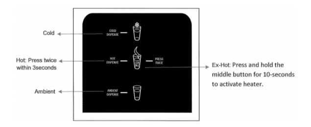
The above picture shows front user interface (UI) and control panel for the *WL3 IT Water Treatment System.*
