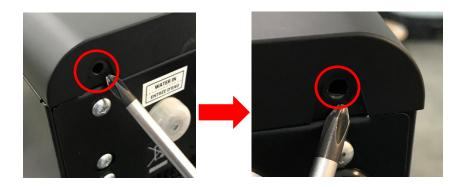
With cover removed, locate and remove the two screws on the backside of the front panel. Then locate and remove the three screws holding the Firewall in place. Tower models will require the lower front panel be removed as well before continuing.
