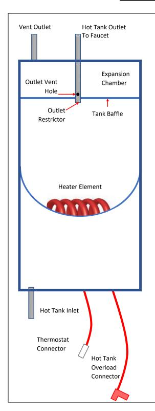
All *Waterlogic* Hot Tanks have a built in Vent or Expansion Chamber in the top of the tank except for WL270 (GF) units.
