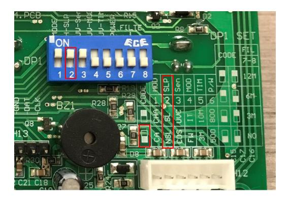
To <u>DISABLE</u> the energy saver, DIP #2 must be switched from ON to OFF (Down position), as per the legend printed on the board. This will enable the hot tank to cycle continuously. All units come with Sleep Mode enabled.
