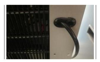
Route the four connections of the IR Module cable through the hole with grommit into the interior of the machine. Leave the other end hanging for now. It will be connected to the IR Module later.
