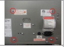
Locate protective metal box on rear of Hot Tank. Push down on top of metal box to access thermostat and overload
