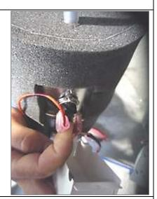
Reattach the metal box by depressing the top flap of the metal box so it snaps back into its original position on the Hot Tank.
