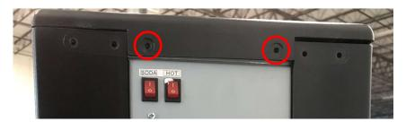
Next, remove the two screws holding the front panel to the frame.
