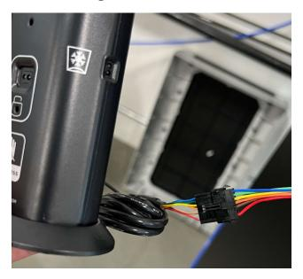
Remove the adhesive backing on the underside of the Touchless Module and firmly press the module down over the hole with the wires tucked inside.
