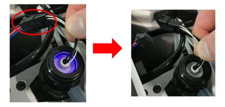
3. Now simply pull the bulb out of the module, replace with a new bulb, and reconnect the wire. Replace the top cover and screws.
