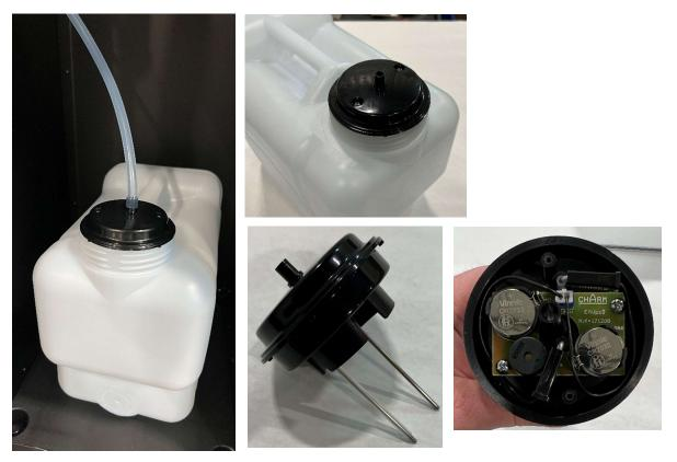
As water collects in the drip tray, it is directed down into this collection tank. Once the tank is ready to be emptied, the level sensor will trigger the alarm built into the cap of the tank. It will **chime for 10 seconds, every 10 seconds** until the tank has been emptied and set back in place.
