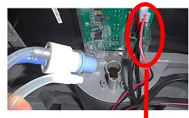
8. Unclip the White, Red and Black wire connectors from PCB to allow Front Cover to be removed.
