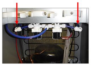
8. Turn outlet fittings outward to avoid water spilling onto the Compressor.
