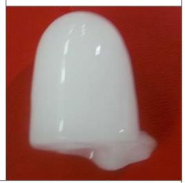
12 proper size and shape ice cubes should be produced every 11-12 minutes once ice making starts. Time and inspect ice shape and size to ensure ice making process is within proper tolerance or sensors could be out of calibration.
