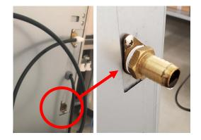
2. The provided drain kit consists of the Molded Drain Line, 3 worm gear clamps, and one female ¾" NPS x 1" Barb fitting that will accept ¾" NPS x ½" CTS.
