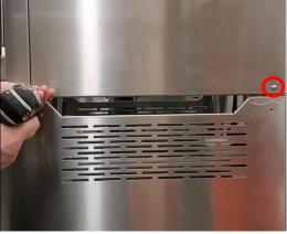
2. Secure the Support Bracket to the base using the screws provided with the bracket. Using the screws from the side panel that were set aside, secure the Support Bracket to the ice machine.
