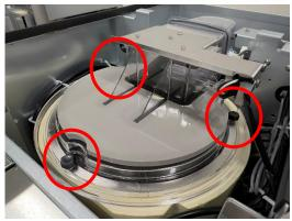
5. Facing the unit, remove the ice dispense auger components from the ice hopper and set them aside. There is the main auger, and a smaller piece that slides into a guide plate inside the hopper. Remove this smaller piece as well.
