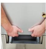
Grab hold of the unit and using your legs, lift the unit. Carefully walk the unit onto the base and set it down with the legs on the base rails.
