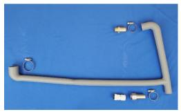
3. Route drain kit from the rear and bottom of the unit and clamp the 1.25" end of the drain kit on to the drip tray port with the provided clamp. Next clamp the 90° end of the drain kit onto the 1" brass barbed fitting on the i30. The dogleg of the drain hose can be connected to any 1" barb fitting using the last clamp to adapt to the desired drain solution.
