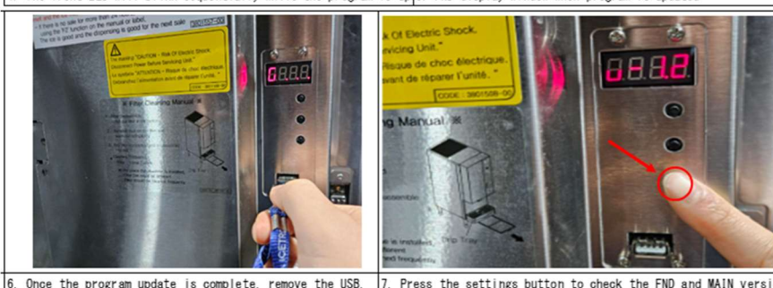
6. Once the program update is complete, remove the USB. 7. Press the settings button to check the FND and MAIN versions.
