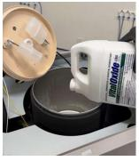
sanitizer). Wipe down the inside of the tank and lid with a lint-free towel. Then, pour ½ gallon of sanitizer into the Ambient Tank and re-install the lid. Connect the unit to power and allow it to fill completely. Sanitizer will make it into the Cold Tank naturally.
