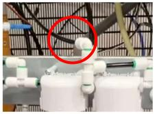
9. **Allow the unit to fill.** Turn the Supply Valve **ON**, and allow the system to begin processing tap water through the RO system and fill the tanks. This can take up to an hour (depending on supply flow).
