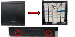
3. Remove the top cover. To do this remove the two screws at the back of the top cover, slide the cover backwards, and lift away from the unit. Shut off the water supply and remove the lid of the Cold tank.
