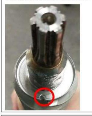
16. seat the spring on the flange with the tip of the spring going through the hole in the flange.
