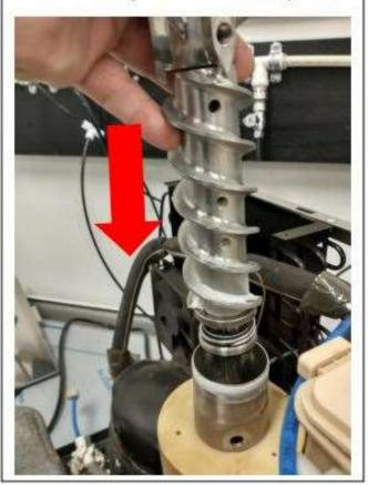
19. using the palm of your hand, press down on the top of the auger, line up the holes in the evaporator with the holes in the extruder and reinsert the bolts.
