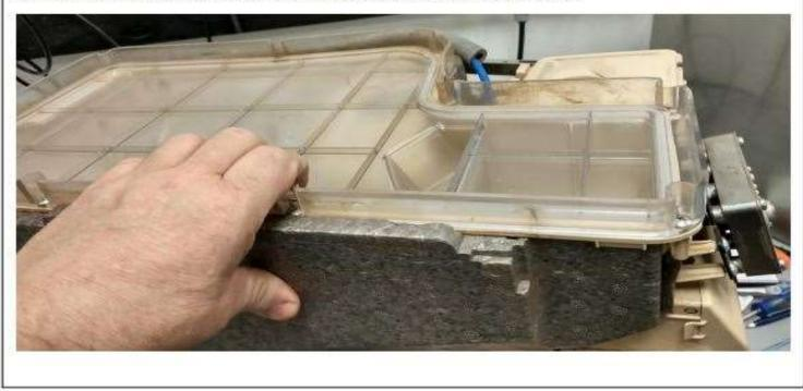
6. remove the bin seal from the top of the evaporator. Clean if necessary and reinstall on the ice bin.
