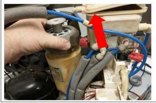
remove 3 12mm bolts. Be sure not to lose the lock washers, spacers, or Orings.
