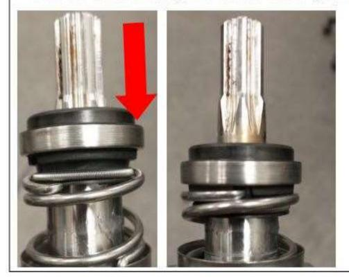
18. slide the auger back into the evaporator
