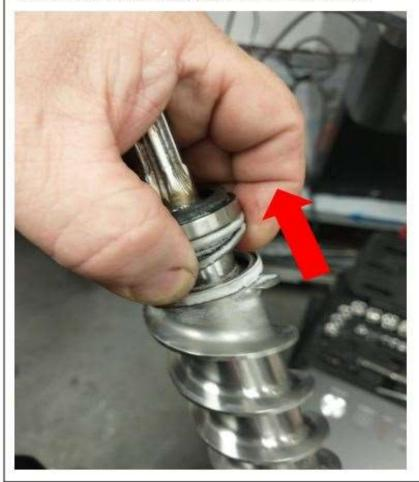
14. clean the area on the auger where the new seal will be located. Lightly coat this area with food grade grease.
