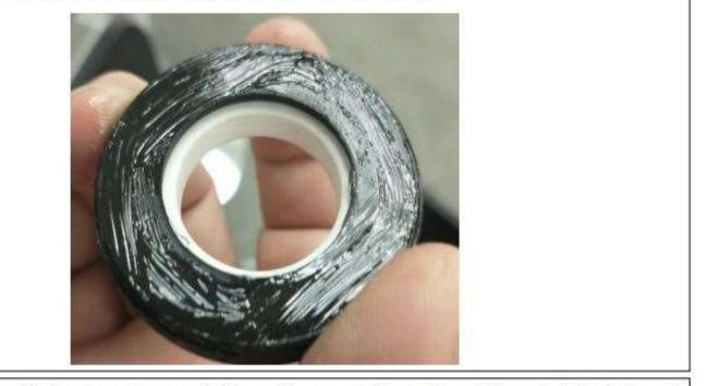
12. place the seal in the evaporator ceramic side up. You may need to gently push the seal into the bottom of the evaporator using the auger.
