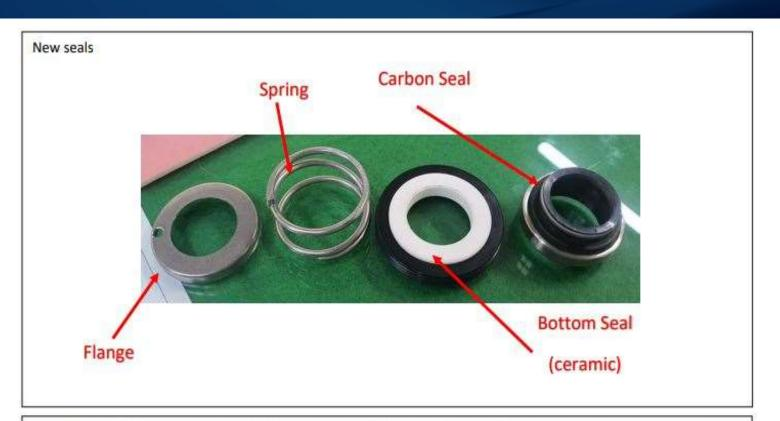
11. lightly coat the rubber portion of the bottom seal with food grade grease. Do not touch or get grease on the ceramic portion of the bottom seal. This can cause the seals to fail prematurely.
