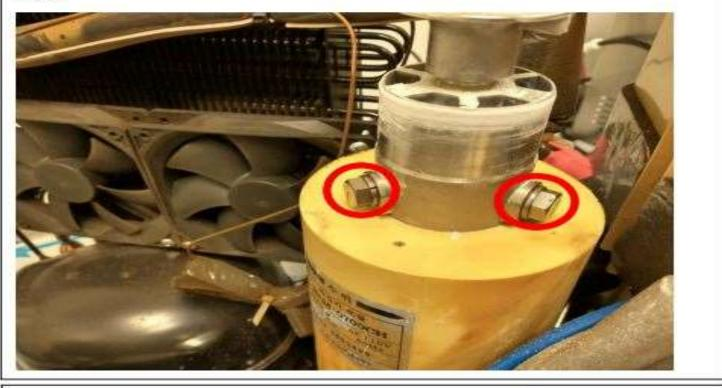
9. once the bolts are removed, pull the Auger out of the Evaporator
