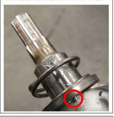
17. slide the carbon seal on the auger with the carbon side facing down and the small spring facing up.
