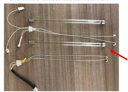
New bulb to be installed; Remove the E-Ballast wire harness. 3. Now, install the glow-start harness onto the new (replacement) bulb. Both long leads connect to one end, and both short leads connect to the other. There is no polarity on the harness, so there is no incorrect lead-to-post combination.
