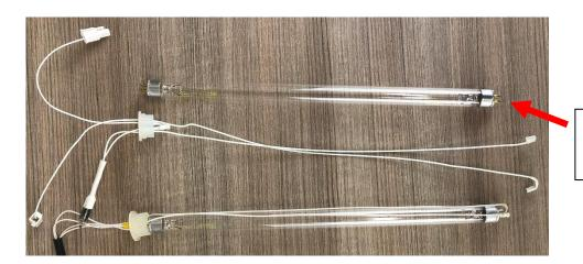
Old bulb to be replaced; Remove the glow-start wire harness.
