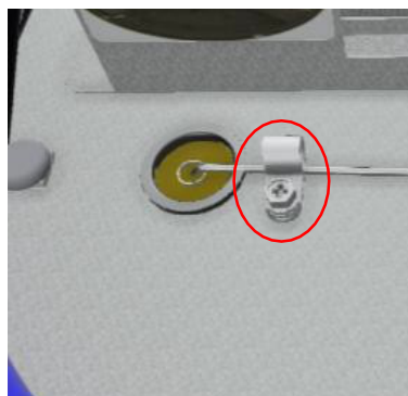
8. Remove screw from harness, and pull the probe out of the bulbwell.
